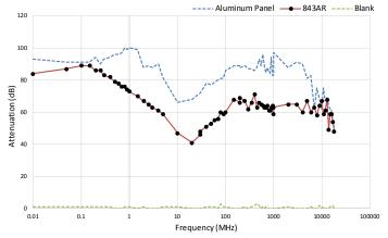
Test performed with a two-coat thickness.
